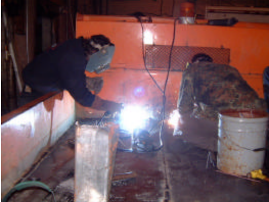
Jim Gallagher and Mick Lee help weld in a new bed liner.
